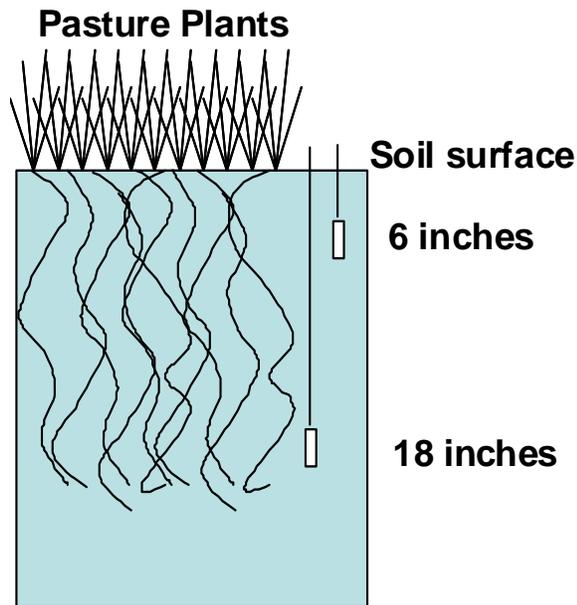
*Irrigation Based on Resistance Block Reading*
